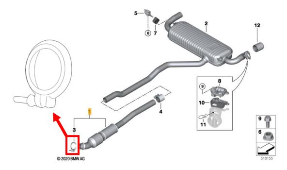
On older models there was a different connection between stock downpipe and link-pipe. Instead of the »V-clamp« mentioned above the »overlapping« connection was used- see schematic bellow. On this vehicles unfortunatelly Akrapovic link -pipe E-BM/SS/6 will not fit because of different joint.
