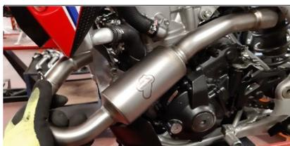
**ENG** First connect the right and left collectors to the bushing and fasten them using the short springs with rubber seal, using the spring puller provided
