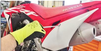
**ENG** Unscrew the fixing screws to the seat and to the side panels right and left side
