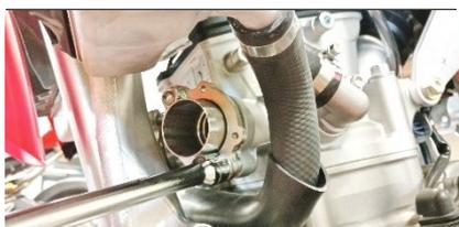
**ENG** Mount the flange on the bushing and place them into the cylinder head, fixing all with the original nuts without tightening
